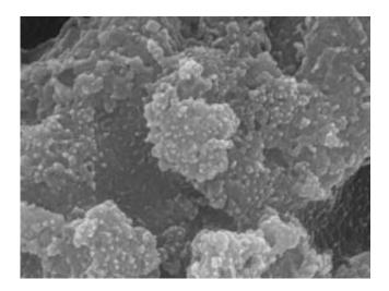
This scanning electron microscope image (magnification x100,000) shows the surface of a porous nickel foam that is peppered with catalytic nanoparticles of cobalt sulfide and nickel sulfide. Credit: A\*STAR Institute of Materials Research and Engineering
