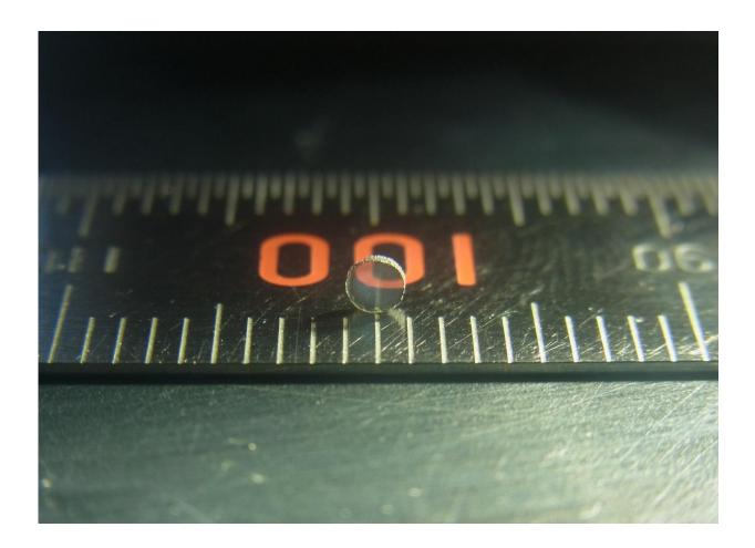
A sample of transparent polycrystalline cubic silicon nitride with a diameter of approximately two millimeters, synthesized at DESY. Credit: Credit: Norimasa Nishiyama, DESY/Tokyo Tech
