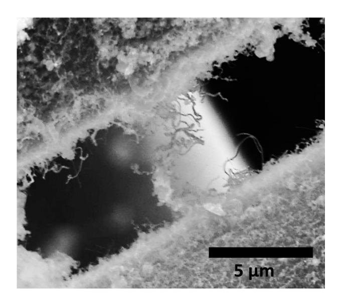
Silicon carbide nanotubes attached to separate silicon carbide fibers, used by NASA, entangle each other in this electron microscope image. The material created at Rice University is intended for a ceramic composite that would make
