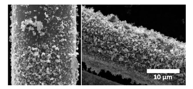
A silicon carbide fiber enhanced with a carpet of 'fuzzy' carbide nanotubes created at Rice University is shown at left. The same fiber with fuzz intact appears at right after researchers burned it with a lighter. Credit: Ajayan Research Group/Rice University
