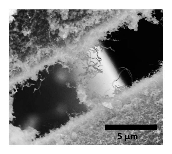
Silicon carbide nanotubes attached to separate silicon carbide fibers, used by NASA, entangle each other in this electron microscope image. The material created at Rice University is intended for a ceramic composite that would make
