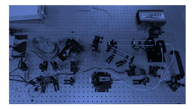
A laboratory setup of instrumentation designed to search for biosignatures on exoplanets using the future Thirty Meter Telescope. The path that light will take through the devices is animated. The equipment is roughly the same size as what would be installed in a telescope, but would be arranged differently. Credit: Caltech/IPAC-TMT
