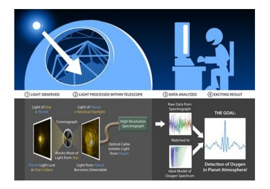
Diagram shows how new technology developed at Caltech will work in the future to help astronomers search for molecular biosignatures on exoplanets. Coronagraphs block a star's light, making orbiting planets easier to see. Highresolution spectrometers would help further isolate a planet's light, and could reveal molecules in the planet's atmosphere. Credit: Caltech/IPAC-TMT
