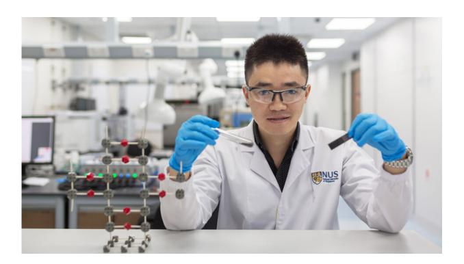
NUS PhD student Mr Liu Wei showing the two-dimensional graphene-like polymer (left), and a piece of carbon paper coated with the novel material (right). Credit: National University of Singapore
