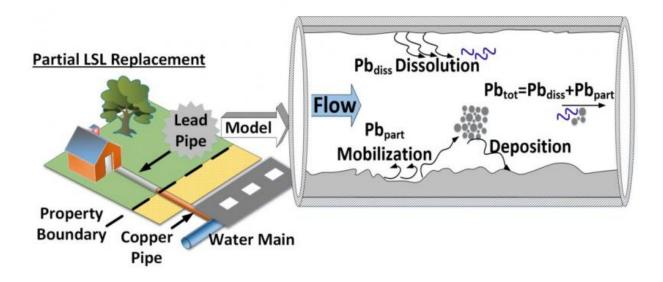
This diagram shows the new model at work: By taking into account a number of factors, including water-use patterns and water chemistry, engineers can predict where lead particles will dislodge and end up in the drinking-water supply during a partial lead service line (LSL) replacement. Credit: Biswas Lab
