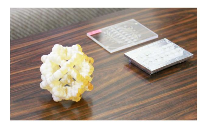
A 3-D printed model of the synthesized ion channel (left) and the highthroughput transmembrane electrical recorder that records the ion current that pases through the channels (right). Credit: Kyoto University iCeMS
