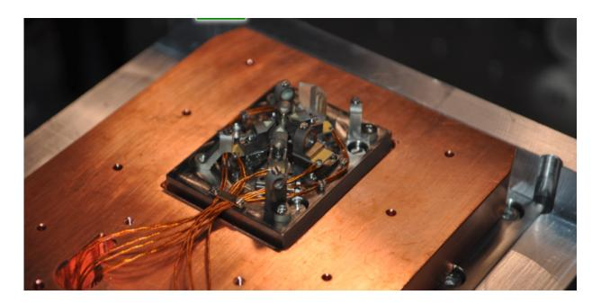
Detail view of the experimental set-up, showing the four mirrors arranged in opposing pairs, each creating an optical resonance chamber. Credit: ETH Zurich
