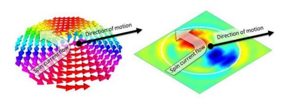
The torque needed to manipulate nanoscale magnetic whirlpools, represented here as red and blue regions with opposite signs, have now been revealed with high-powered synchrotron light. Credit: Reproduced with permission of 2016 American Physical Society
