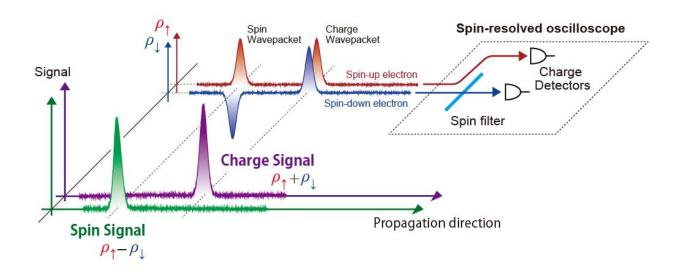
The spin-resolved oscilloscope is established by combining spintronic and plasmonic devices, i.e., a spin filter and time-resolved charge detectors. Credit: Masayuki Hashisaka
