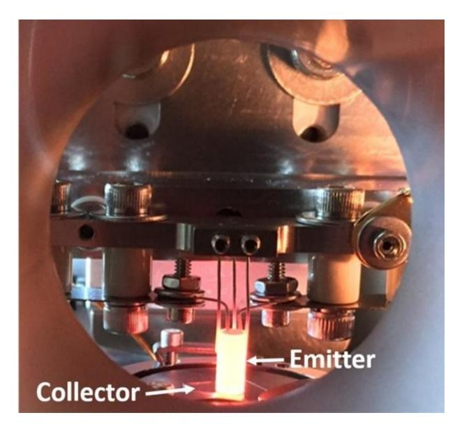
Photograph of the TEC prototype during operation in the Stanford lab. Credit: Elsevier
