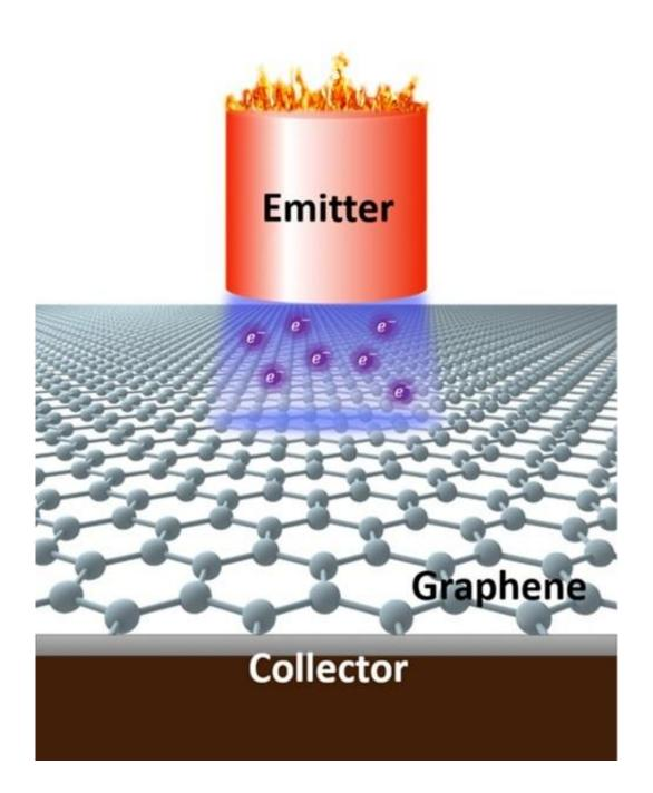
Schematic sketch of the thermionic energy convertor prototype with a graphene collector. Credit: Elsevier
