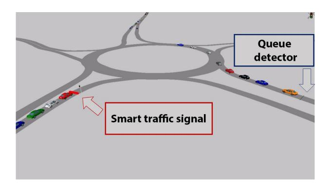
The smart traffic light on one of the roundabout approaches would only be activated or turn red when the queue detector on the other approach road indicates there is a queue. Credit: Mariló Martín-Gasulla et al./UPV
