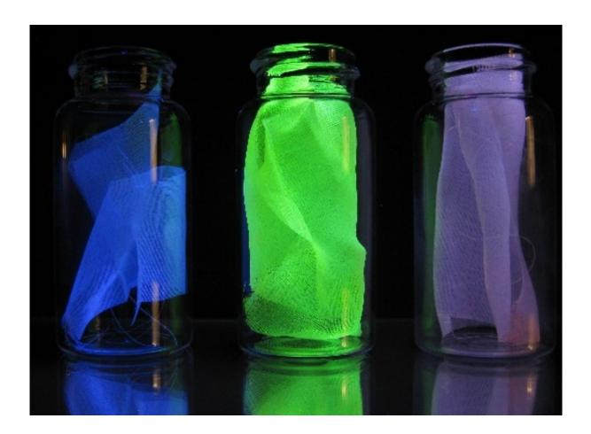
These are examples of the silk used in experiments to detect damage in composites, shown under black light. (Left) Ordinary fibroin of the Bombyx mori silk worm. The observed fluorescence is the result of molecules already present in the protein structure of the fiber. (Middle) Mechanophore-labeled silk fiber fluoresces in response to damage or stress. (Right) Control sample without the mechanophore. Credit: Chelsea Davis and Jeremiah Woodcock/NIST
