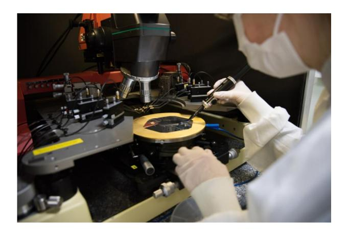
The scientist carefully places the sensors in the probe station and tests them by applying a high voltage using a needle. The team must wear protective equipment to keep the sensor safe from dust and scratches. Credit: Ulysse Fichet/CERN
