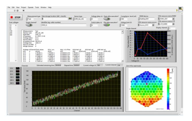
The software shows the current running through each sensor, and the tile made of multiple smaller sensors is shown on the bottom right. Credit: Andreas Maier/CERN
