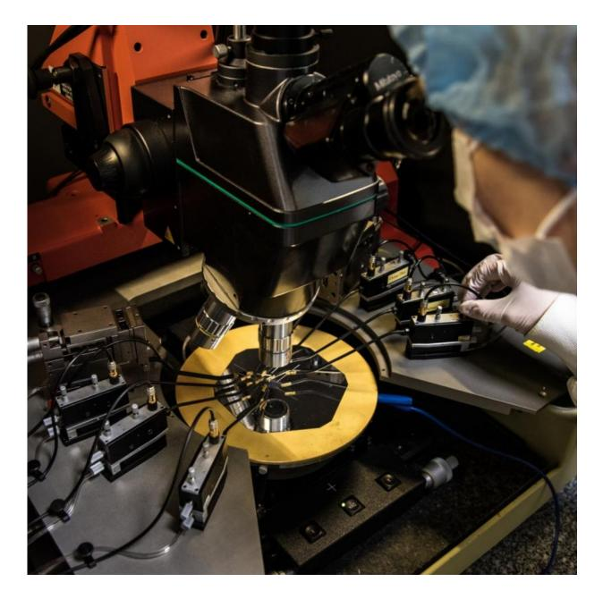
Eva Sicking works on the probe station. She explains: "Currently we use individual probe needles to contact the cell we want to test and all of its direct neighbours, but we're also developing a probe card with many pins below it so we can lower the card and connect all the pins and test all the sensors cells in one go, so we won't need to place each of the eight needles individually.". Credit: Ulysse Fichet/CERN
