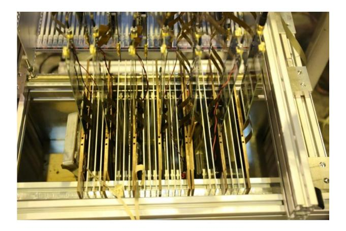
A team of CMS researchers have already tested the first sandwich calorimeter prototype with single particles, but in the upgraded HL-LHC multiple particle collisions will occur at once and hundreds of debris particles will pass through the sensors at the same time. The prototype is based on silicon and dense metals – the image shows the alternating layers of metal and the silicon sensor. The particle beam will run from the left of the image through to the right. Credit: David Barney/CERN
