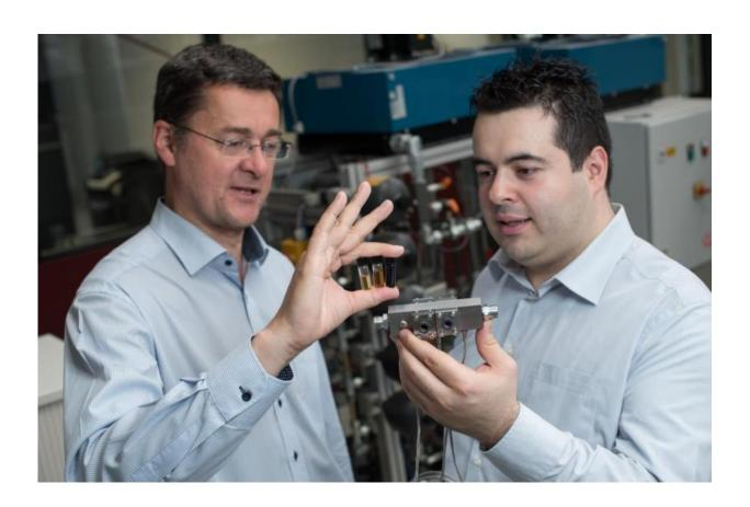
Prof. Andreas Schütze (left) and Dipl.-Ing. Eliseo Pignanelli are showcasing a measuring system at Hannover Messe that continuously monitors oil quality and predicts when an oil change is required. The oil flows through the measuring cell where it is irradiated with infrared light. The oil samples in the bottles indicate how oil visibly ages: the bottle on the left contains new oil. Credit: Oliver Dietze
