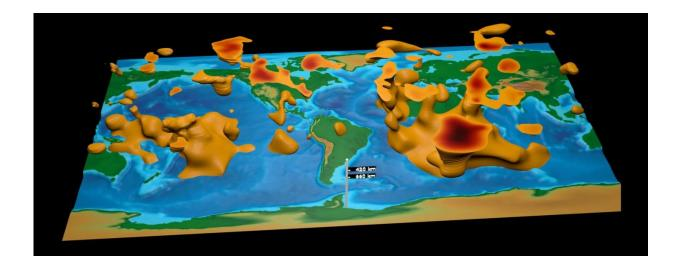
This visualization is the first global tomographic model constructed based on adjoint tomography, an iterative full-waveform inversion technique. The model is a result of data from 253 earthquakes and 15 conjugate gradient iterations with transverse isotropy confined to the upper mantle. Credit: David Pugmire, ORNL
