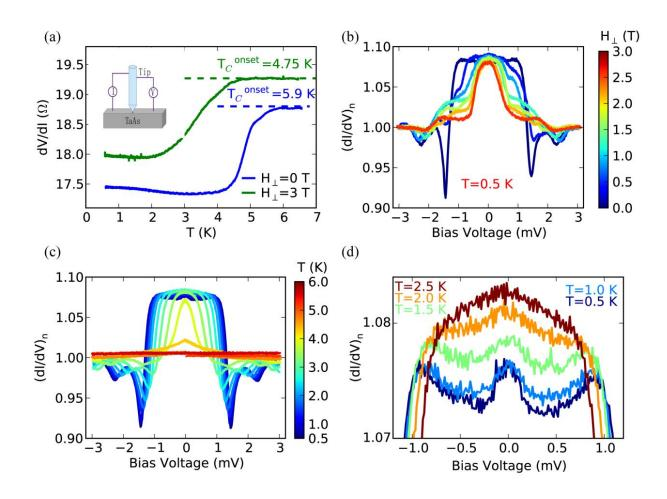
(a) Temperature dependence of zero-bias PC resistance showing typical superconducting transition. Inset: Schematics of the PCS measurement configuration. (b) Normalized dI/dV spectra at 0.5 K under different out-of-plane magnetic fields. The navy blue line denotes zero field measurement. (c)
