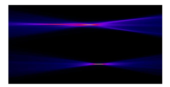
A profile of the focused X-ray beam, without (top) and with (bottom) the corrective lens. Credit: Frank Seiboth, DESY
