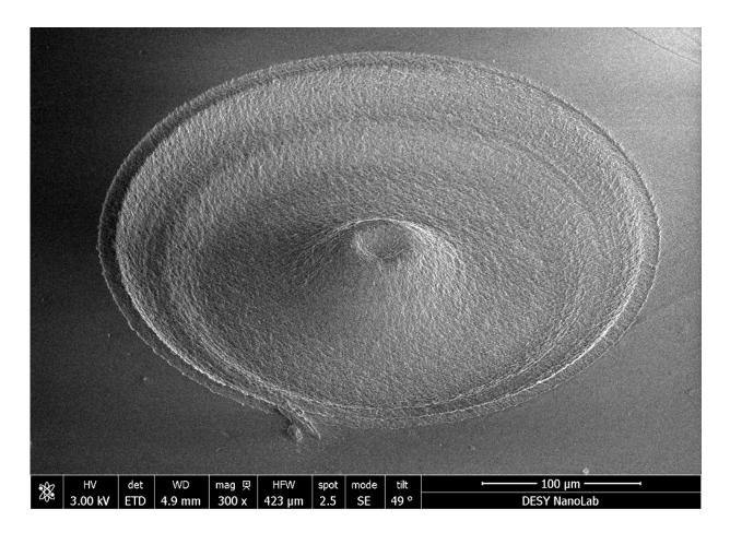
The X-ray spectacles under an electron microscope. Credit: DESY NanoLab
