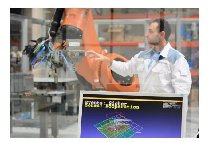
Safety zones: The display shows the different zones. In the yellow zone, robots and humans collaborate, with the robot moving significantly slower in this zone. Credit: Fraunhofer IWU
