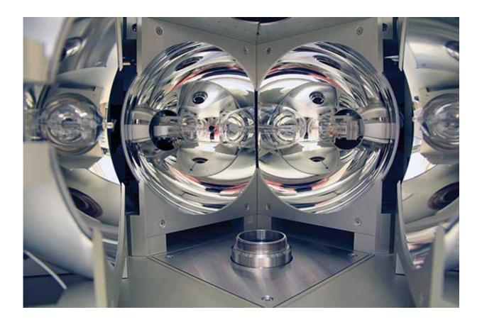
Four semi-spherical reflectors focus light energy from highpowered halogen bulbs onto the material, which is suspended over the port in the center. Credit: Ames Laboratory
