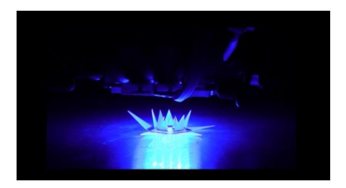
Inspired by origami, North Carolina State University researchers have found a way to remotely control the order in which a two-dimensional (2-D) sheet folds itself into a three-dimensional (3-D) structure.
