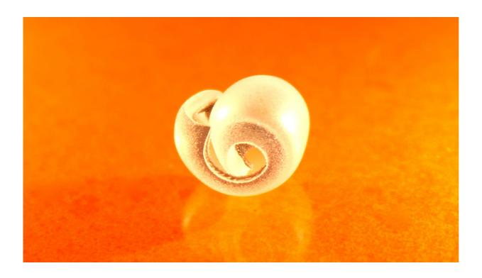
Researchers at North Carolina State University have developed a technique that uses light to get flat, plastic sheets to curve into shapes such as spheres, tubes or bowls. Credit: Amber Hubbard
