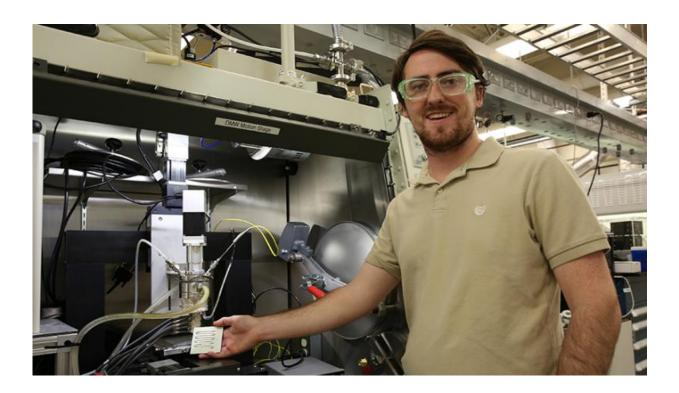
Lawrence Livermore scientist Luke Thornley helped engineer the semisolid metal, a bismuth-tin mixture, that can be extruded through the nozzle of a specially designed 3D printer. Credit: Kate Hunts/LLNL
