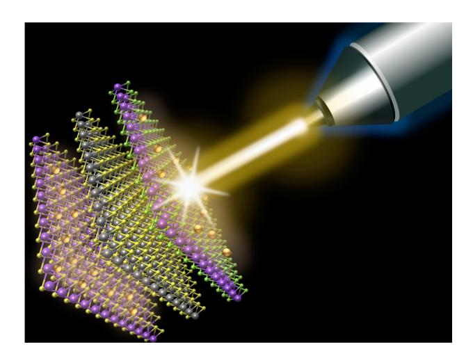
Illustration of laser beam triggering quantum movement of electrons between top and bottom layers, bypassing middle layer. The new tri-layer material from KU's Ultrafast Laser Lab material someday could lead to next-generation electronics. Credit: Frank Ceballos, University of Kansas
