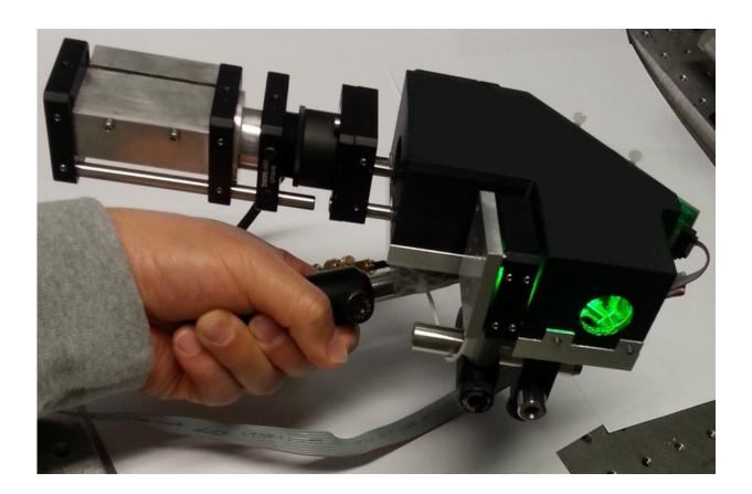
This handheld device for transmitting and receiving quantum cryptographic keys was built from off-the-shelf components. The device could be miniaturized for use in a mobile device. Credit: Iris Choi, Oxford University
