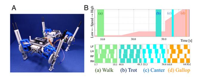
A The quadruped robot, Oscillex 3. B Reproduced changes in step (gait transition phenomenon). (Top) Change in the parameter related to speed (Bottom) The colors represent periods when a leg senses weight on the corresponding leg. The gait transition was demonstrated from walk to trot, to canter, to gallop. Credit: Akio Ishiguro
