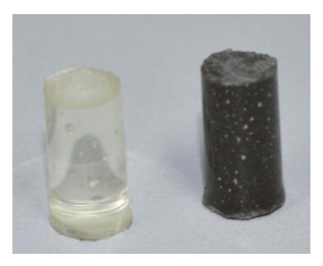
This is a transparent piece of epoxy, left, compared to epoxy with e-waste reinforcement at right. A cryo-milling process developed at Rice University and the Indian Institute of Science simplifies the process of separating and recycling electronic waste. Credit: Chandra Sekhar Tiwary/Rice University
