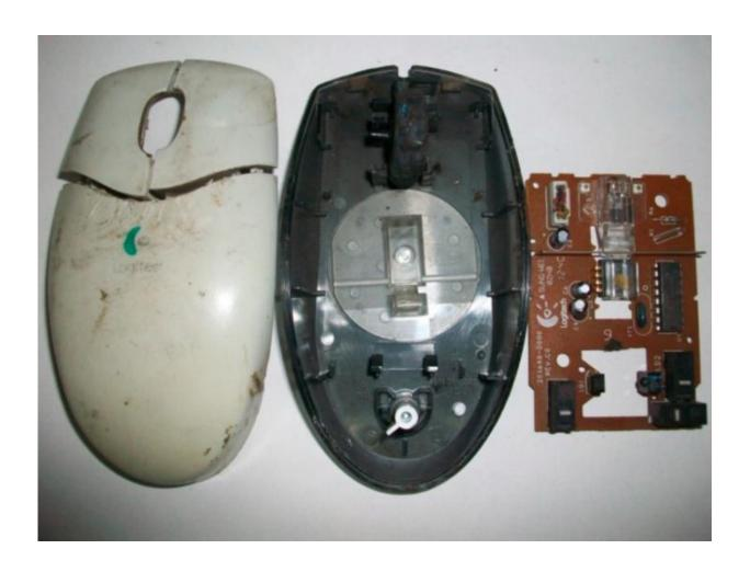
Circuit boards from electronics, like computer mice, can be crushed into nanodust by a cryo-mill, according to researchers at Rice University and the Indian Institute of Science. The dust can then be easily separated into its component elements for recycling. Credit: Chandra Sekhar Tiwary/Rice University
