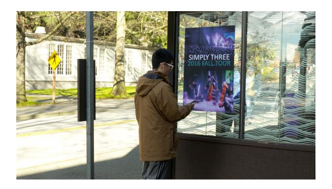
UW engineers used FM radio signals to broadcast music and data notifications from a Simply Three band poster at a Seattle bus stop to a smartphone. An antenna made of copper tape was embedded on the back of the poster. Credit: University of Washington
