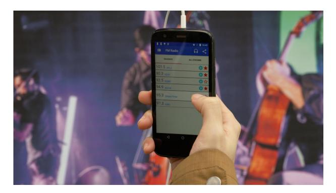
The FM backscattering system encodes audio or data on top of a regular FM broadcast but uses an unoccupied frequency in the FM radio band to send that information to a smartphone or car radio receiver. Credit: University of Washington
