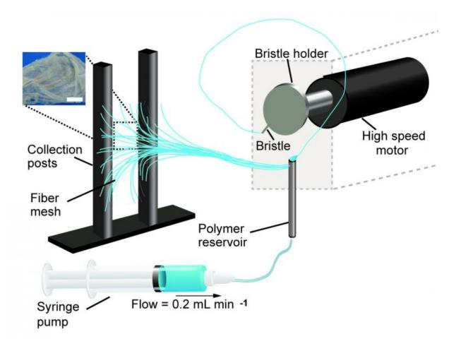
A schematic of the pull spinning apparatus with a side view illustration of a fiber being pulled from the polymer reservoir. The pull spinning system consists of a rotating bristle that dips and pulls a polymer jet in a spiral trajectory. Credit: Leila Deravi/Harvard University
