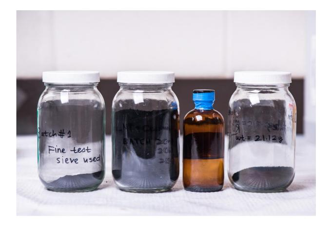
These jars show variations of a Kansas State University-patented liquid polymer that looks like water and has the same density and viscosity as water. The polymer becomes a ceramic when heated and can be mass-produced. Credit: Kansas State University
