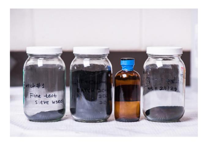
These jars show variations of a Kansas State University-patented liquid polymer that looks like water and has the same density and viscosity as water. The polymer becomes a ceramic when heated and can be mass-produced. Credit: Kansas State University
