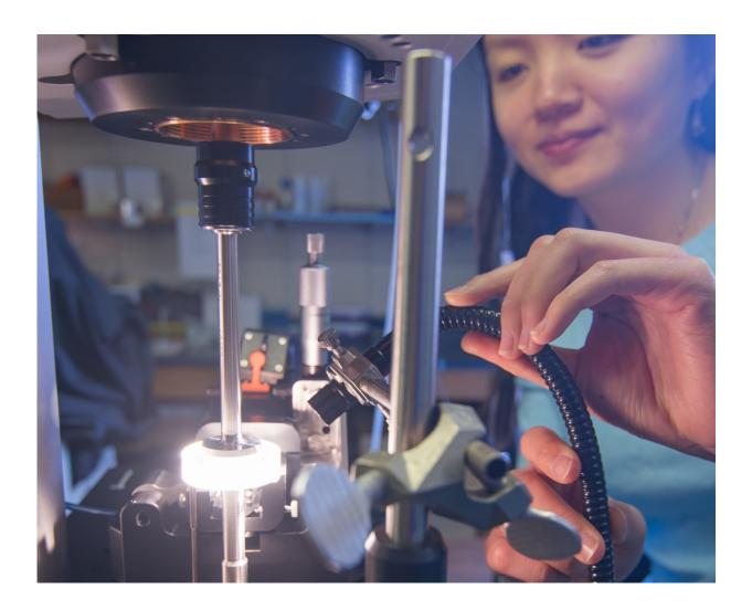
The rheometer developed by UCSB's Helgeson Lab and instrumentation manufacturer Anton Paar Credit: Scott Condon
