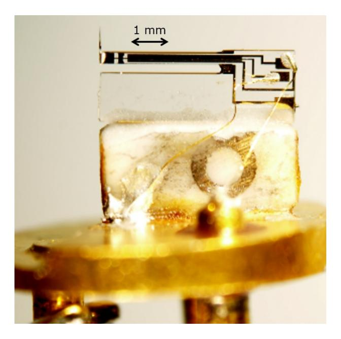
Sensor inside the force microscope. Credit: Vienna University of Technology
