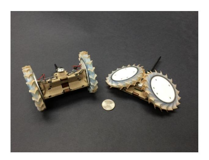
Pop-Up Flat Folding Explorer Robot (PUFFER) was inspired by an origami design. This little robot could be used as a scout for larger rovers, going places that would be risky or hard to reach. Credit: NASA/JPL-Caltech
