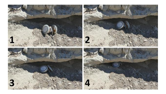
PUFFER crawls under a ledge during field testing. The advantage of its small size and foldable body is that the bot can wedge itself into small spaces. That could be useful on the rugged terrain of other planets. Credit: NASA/JPL-Caltech
