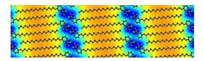
Calculated differential electrical potential induced by a supramolecular lattice of MBB-2 on graphene. The supramolecular lattice is superimposed for clarity. The electrical potential is periodically modulated, with negative values in the region below the molecular heads. Carbon atoms are shown in grey, hydrogen in white, nitrogen in red, fluorine in light blue and chlorine in green. Credit: Lohe
