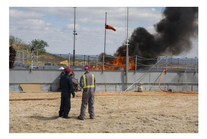
The Flame Refluxer prototype is tested in the burn pan at the Joint Maritime Test Facility in Mobile, Ala., part of tests conducted between March 13-17, 2007. Developed by fire protection engineering researchers at Worcester Polytechnic Institute (WPI), the device designed to burn off oil spills more completely. It transmits heat from an oil fire into the oil to superheat it and make the fire hotter, more productive, and cleaner. Credit: Worcester Polytechnic Institute
