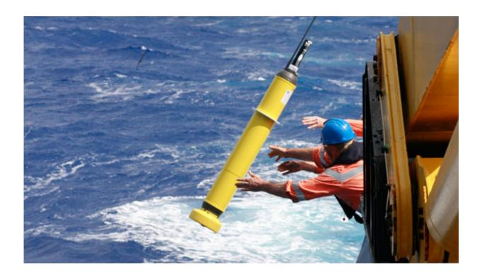
The deployment of an Argo float off a research vessel. Data collected from Argo floats were used to validate a new estimate of ocean heat content. (Image courtesy of the Australian Commonwealth Scientific and Industrial Research Organization.)
