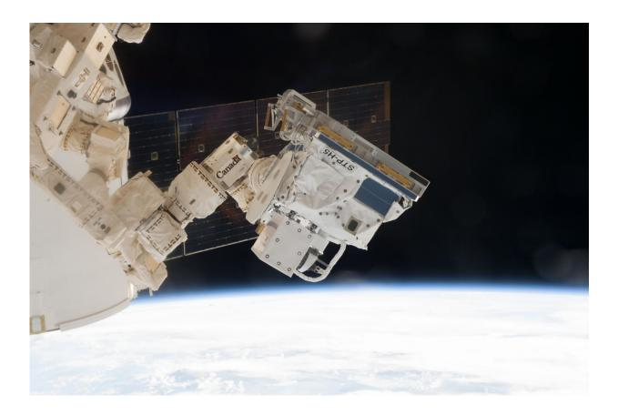
This image shows the Defense Department's experiment pallet, STP-H5, hanging at the end of Canada's robotic arm during installation on the outside of the International Space Station. Credit: NASA
