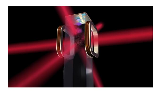
Artist's concept of an atom chip for use by NASA's Cold Atom Laboratory (CAL) aboard the International Space Station. CAL will use lasers to cool atoms to ultracold temperatures. Credit: NASA
