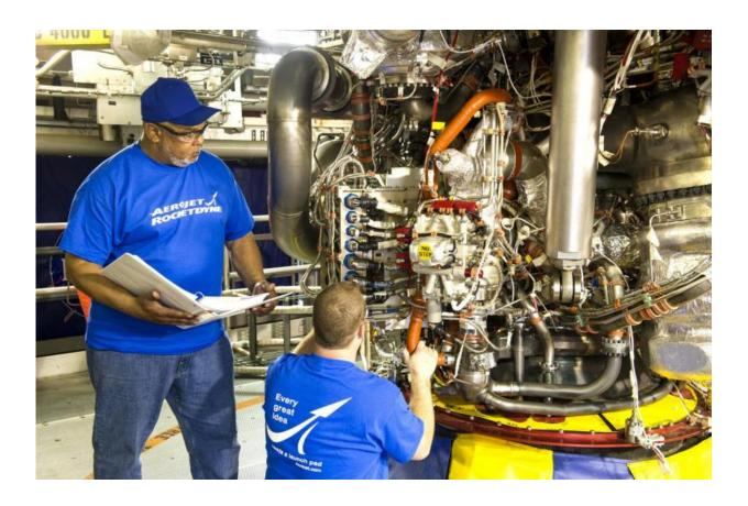
Aerojet Rocketdyne technicians inspect the engine controller that will be used for the first integrated flight of NASA's Space Launch System and Orion in late 2018. The engine controller was installed on RS-25 development engine no. 0528 for testing at Stennis Space Center on the A-2 Test Stand on March 23, 2017. The RS-25 engine, with the flight controller, was test fired for a full-duration 500 seconds. Credit: NASA/SSC
