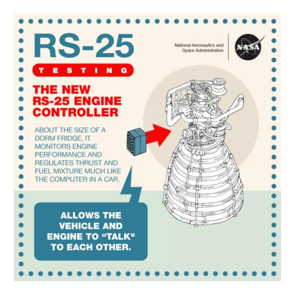
RS-25 new engine controller. Credit: NASA/SSC
