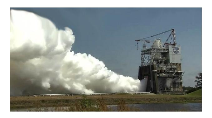
NASA engineers conduct a test of the first RS-25 engine controller that will be used on an actual Space Launch System flight on the A-2 Test Stand at Stennis Space Center on March 23, 2017. The RS-25 engine, with the flight controller, was test fired for a full-duration 500 seconds. Credit: NASA/SSC
