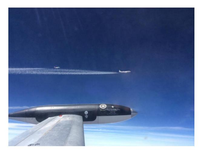
NASA's HU-25C Guardian aircraft flies 250 meters behind the agency's DC-8 aircraft on May 14, 2014, before it descends into the DC-8's exhaust plumes to sample ice particles and engine emissions. Credit: National Research Council of Canada
