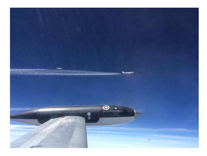
NASA's HU-25C Guardian aircraft flies 250 meters behind the agency's DC-8 aircraft on May 14, 2014, before it descends into the DC-8's exhaust plumes to sample ice particles and engine emissions. Credit: National Research Council of Canada
