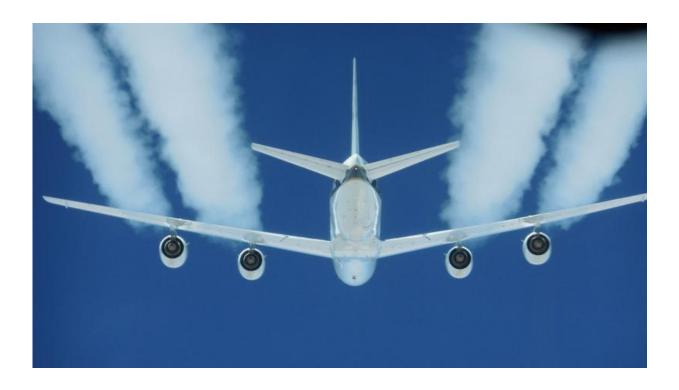
The DC-8's four engines burned either JP-8 jet fuel or a 50-50 blend of JP-8 and renewable alternative fuel of hydro processed esters and fatty acids produced from camelina plant oil. Credit: NASA/SSAI Edward Winstead
