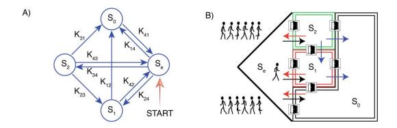
(Left) The four states of the atom correspond to (right) the four rooms of a maze. The random nature of tunneling electrons in and out of an atom simulates the movement of people between rooms of the maze, and can optimize the solutions to certain maze problems. Credit: Fresch et al. ©2017 American Chemical Society
