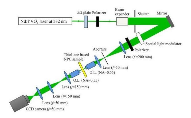
Optical setup for coaxial holographic digital data page recording. Credit: University of Electro Communications
