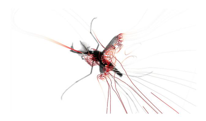
Culex mosquitoes exhibit unusual aerodynamic mechanisms. Streamlines (red) show a vortex along the trailing edge that gives the insects a boost in lift force. Credit: Bomphrey/Nakata/Phillips/Walker
