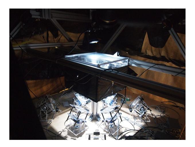
Dr Nathan Phillips constructed a specialised arena with eight powerful infra-red high-speed cameras recording at 10,000 frames per second to capture the wing movements of mosquitoes in flight. Credit: Bomphrey/Nakata/Phillips/Walker
