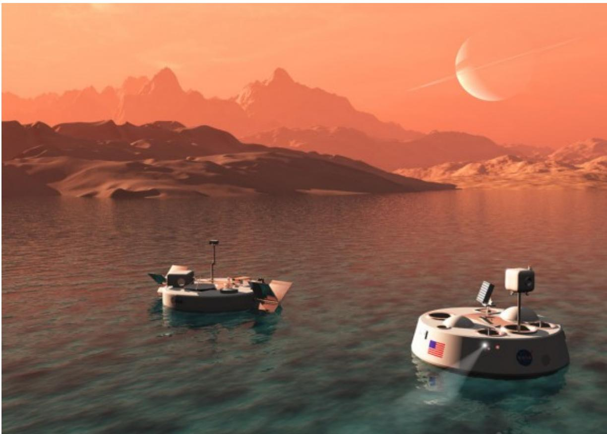
On the left is TALISE (Titan Lake In-situ Sampling Propelled Explorer), the ESA proposal. This would have its own propulsion, in the form of paddlewheels.
