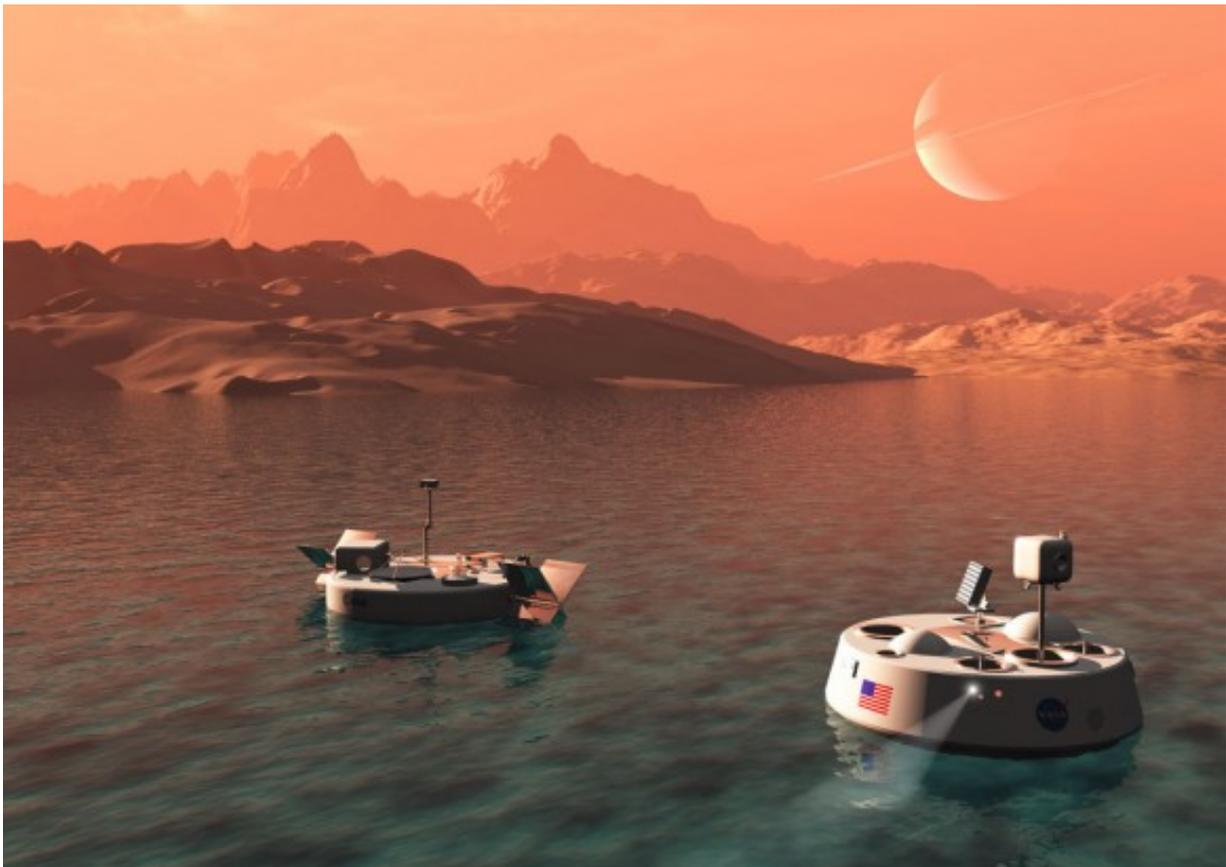
On the left is TALISE (Titan Lake In-situ Sampling Propelled Explorer), the ESA proposal. This would have its own propulsion, in the form of paddlewheels. Credit: bisbos.com
