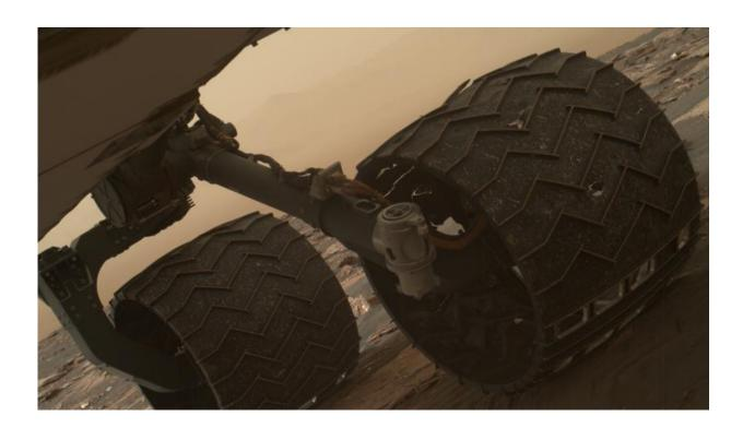
Two of the raised treads, called grousers, on the left middle wheel of NASA's Curiosity Mars rover broke during the first quarter of 2017, including the one seen partially detached at the top of the wheel in this image from the Mars Hand Lens Imager (MAHLI) camera on the rover's arm. Credit: NASA/JPL-Caltech/MSSS
