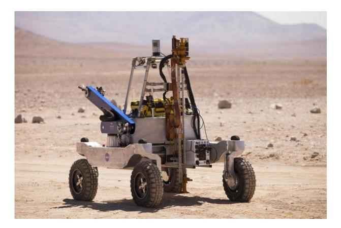
The rover in its mobile configuration with drill raised and visible at the front, arm stowed, and instruments closed. Credit: NASA/CampoAlto/V. Robles
