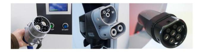
No common standard: CHAdeMO, CCS and Tesla Supercharger plugs. Credit: CHAdeMO: C-CarTom; CCS: Hadhuey; Tesla: Paul Sladen, CC BY-SA
