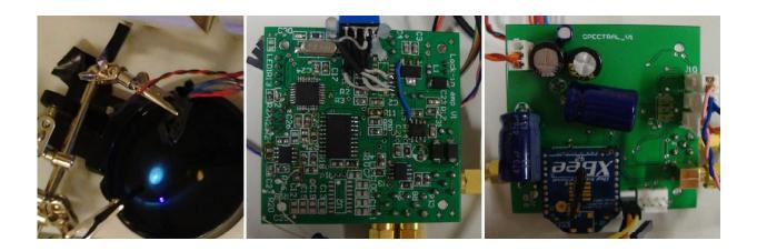
Researchers developed a device that uses florescence from oil (left) to detect its presence and identify the type of oil. The small and simple device incorporates inexpensive electronic components (right). Credit: Oscar Sampedro, Universidade de Vigo.
