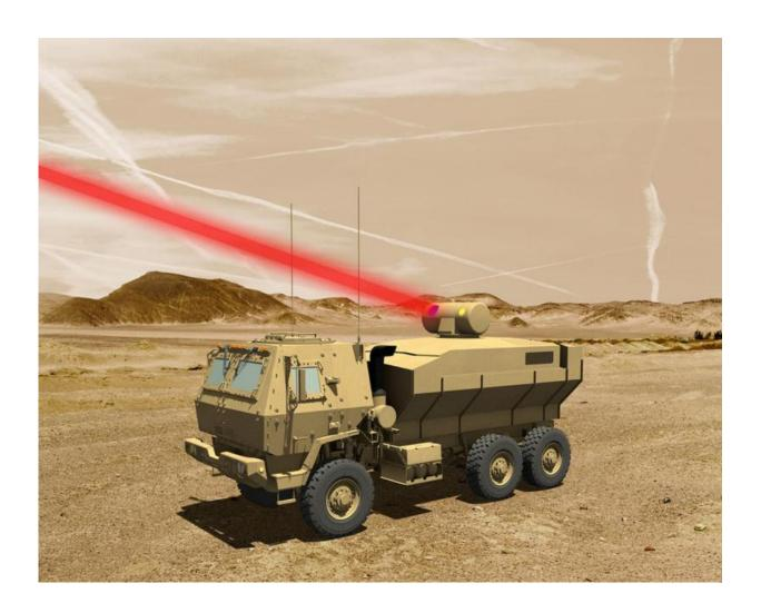
A rendering of a truck mounted 60 kW laser weapon system for tactical U.S. Army vehicles. Credit: Lockheed Martin
