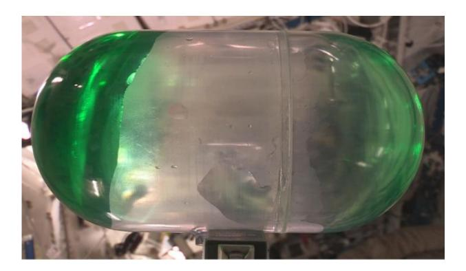
Tank from an earlier Slosh experiment aboard the International Space Station. The tanks for this investigation are similar. Credit: NASA
